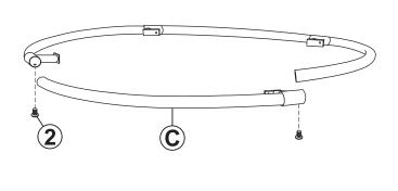
Align the mounting holes on the four Safety Rings (C) and loosely secure using four M6x10mm Bolts (2).
