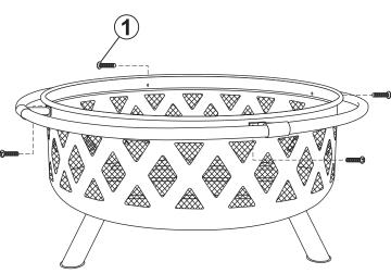
Carefully guide the assembled ring up from the bottom of the fire bowl, align the safety ring brackets with the mounting holes in the fire bowl, and loosely fasten it using four M6x25mm Bolts (1) and M6 Nuts (3).
