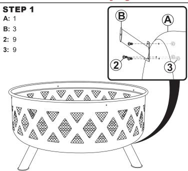
Ensuring the flat edge of the leg is facing outward, align Leg (B) with the bottom of Fire Bowl (A) and loosely fasten using three M6x10mm Bolts (2) and M6 Nuts (3). Repeat to attach the remaining two legs.
