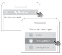
**4.** Follow app instructions to complete the setup. The Signal LED should turn solid on, indicating successful connection to your router.
