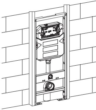
**2 Dry Fit Outlet Pipe & Inlet Pipe**
