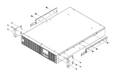
Position the guide screw on the back of the rackmount rails into the rear rack square holes to temporarily support the rails in place.
