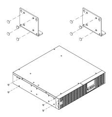
Step 2: Attach the base stands and attach the dust covers
