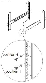
Step 5: Place and secure the UPS on the rails
