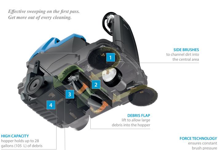
Force Technology, standard on every machine, keeps the brush in contact with the floor at all times. It automatically adjusts brush pressure over uneven surfaces or protrusions, producing a uniform cleaning result.
