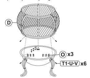
Loosely fasten three Brackets (O) to the bottom bowl using three 1/4"x3/4" Bolts (T1), Washers (U), and Nuts (V).
