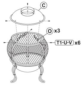
Loosely fasten three Brackets (O) to the screen using three 1/4"x3/4" Bolts (T1), Washers (U), and Nuts (V).
