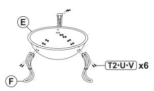
Securely fasten each Leg (F) to Bottom Bowl (E) using two 1/4"x5/8" Bolts (T2), Washers (U), and Nuts (V).
