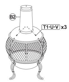
Securely fasten Main Flue (B2) to the bowl top using three 1/4"x3/4" Bolts (T1), Washers (U), and Nuts (V).
