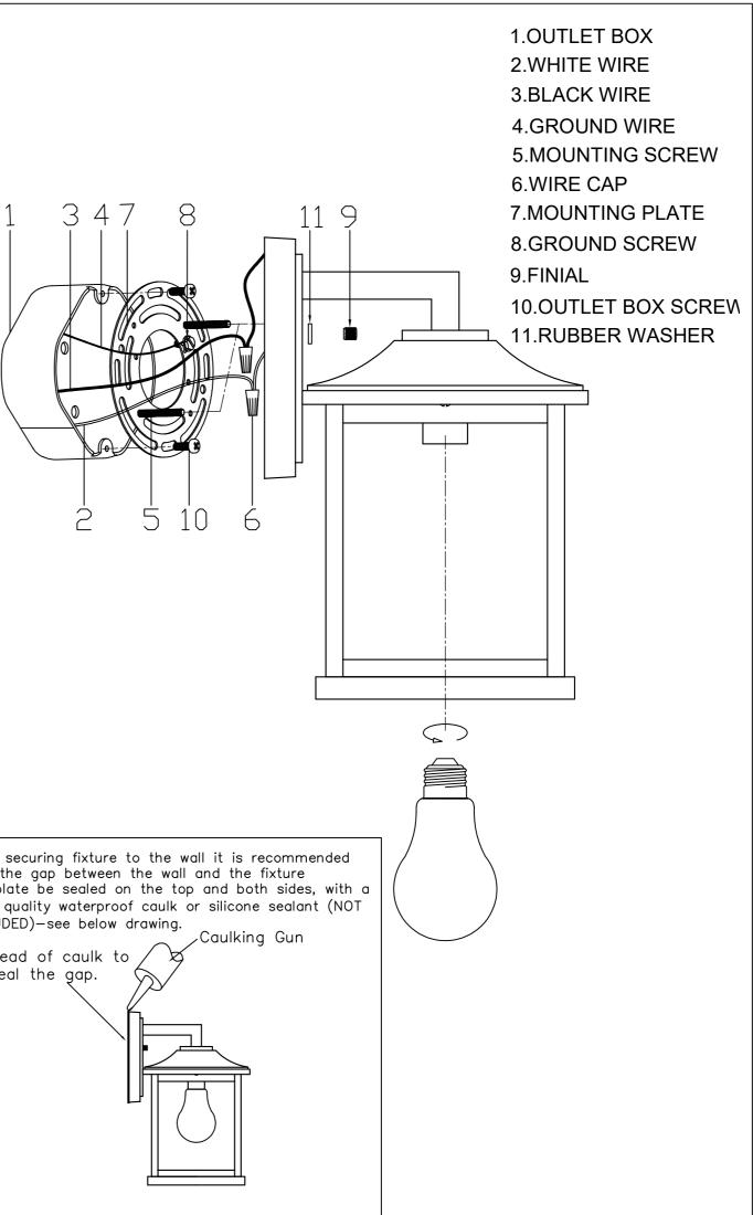
After securing fixture to the wall it is recommended that the gap between the wall and the fixture backplate be sealed on the top and both sides, with a good quality waterproof caulk or silicone sealant (NOT INCLUDED)-see below drawing.
