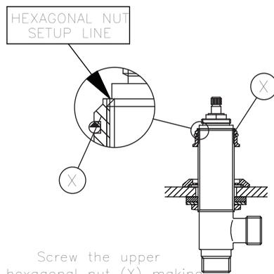
Screw the upper hexagonal nut (X) making sure to place it at the end of the body's thread (HEXAGONAL NUT SETUP LINE).
