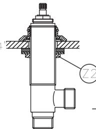
Place (H) the square disc in the right position before screwing the underside hexagonal brass fixing nut (Z2).
