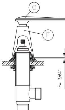
Assemble the handle set (G) screwing the cap (F), placing it in the correct position.
