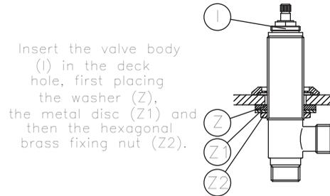
Insert the valve body (I) in the deck hole, first placing the washer (Z), the metal disc (Z1) and then the hexagonal brass fixing nut (Z2).
