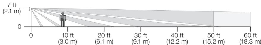
\* Sensor mounting shown at 7 ft (2.1 m). Mounting height should be between 6 ft and 8 ft (1.6 m and 2.4 m).
