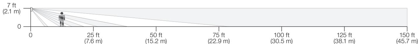
\* Sensor mounting shown at 7 ft (2.1 m). Mounting height should be between 6 ft and 8 ft (1.6 m and 2.4 m) and centered within hallway.
