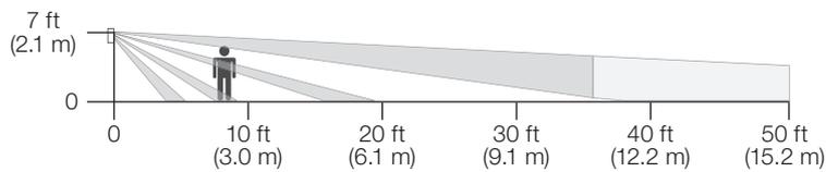
\* Sensor mounting shown at 7 ft (2.1 m). Mounting height should be between 6 ft and 8 ft (1.6 m and 2.4 m).
