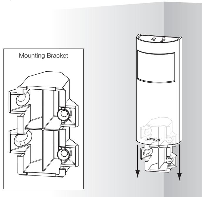
Figure C. Flexible Mounting Armature
