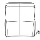
STEP 2 - Connect the connector from motor to the power cord and transformer
