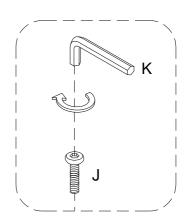
Using bolt (J) attach part (9) into part (2) with Hex key (K) as per diagram.
