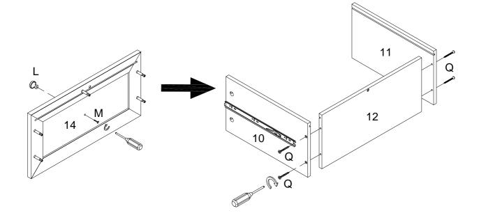
Using handle bolt (M) secure handle (L) to part (14) ,then using screw(Q) attach parts (10,11) to part (12) with Philips head screwdriver as per diagram.
