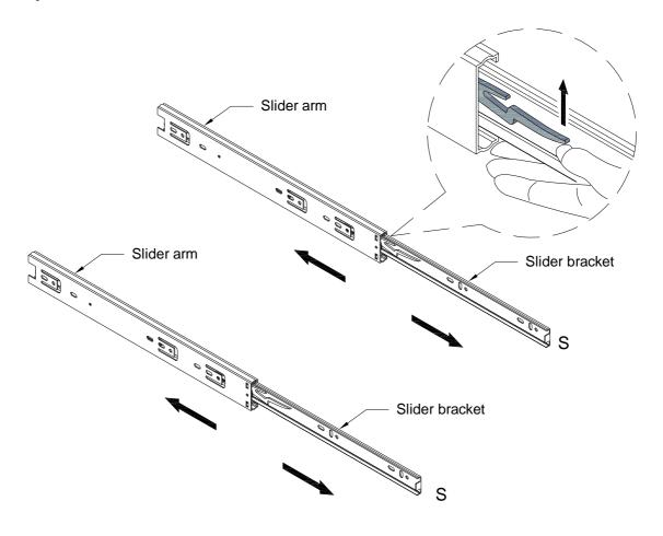
Pick up the slider arm (S) and separate the slide runner for the following Steps. Extend the slide runner all the way forward,press the plastic release lever of the slider arm up and pull the slide runner complete out .
