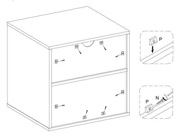
Using screw (N) secure plastic wedge (P) with Philips head screwdriver as per diagram.
