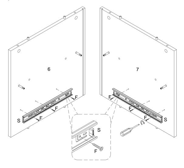
Using screw (F) attach drawer slider (S) to parts (6,7) with Philips head screwdriver as per diagram.
