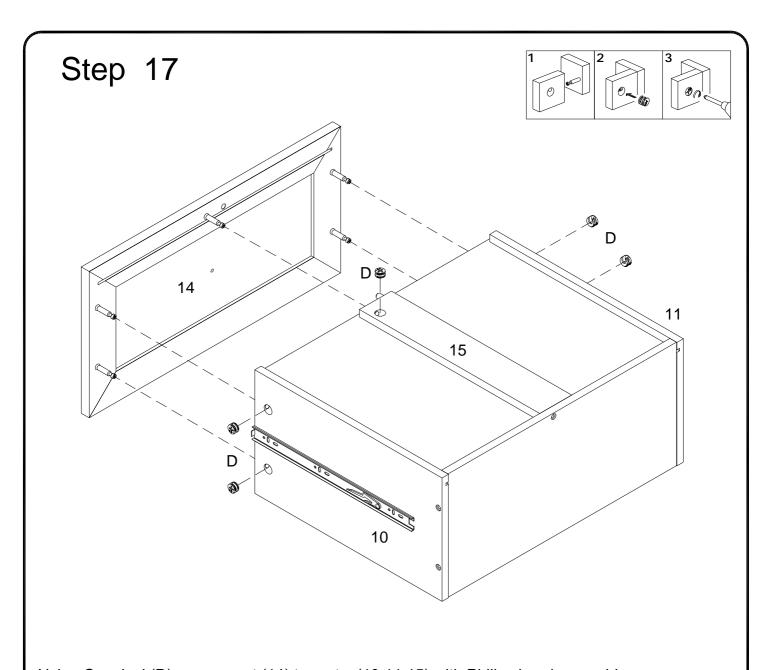
Using Cam lock(D) secure part (14) to parts (10,11,15) with Philips head screwdriver as per diagram.
