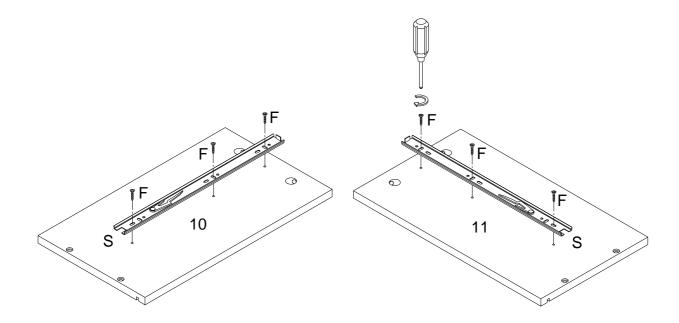
Using screw (F) attach drawer slider (S) to parts (10,11) with Philips head screwdriver as per diagram.
