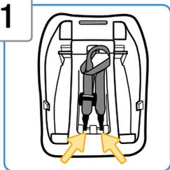
**Remove Lower Anchor Belt from Storage Attachments**
