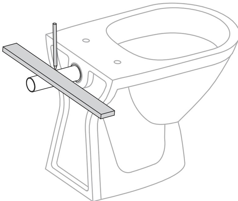
3. Carefully measure between your marks, this distance will be cut off the bald end. Add  $\frac{15}{64}$ " to measurement before cutting, leaving a small cushion for error.
