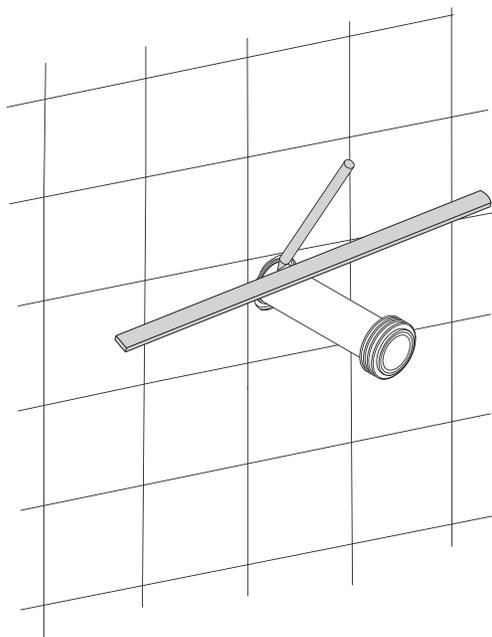
2. Insert tube into bowl and mark as shown.
