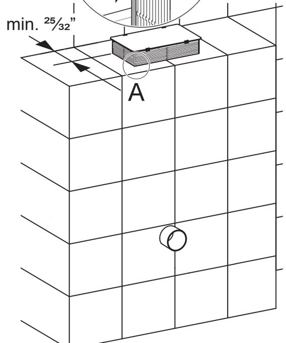
1. Insert tube into wall and mark as shown.
