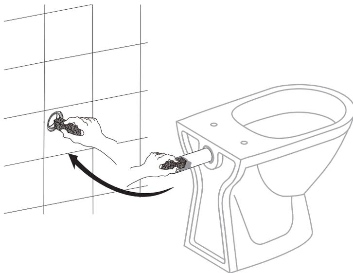
6. Ensure the bowl is level and install. Caulk and seal around the bowl.
