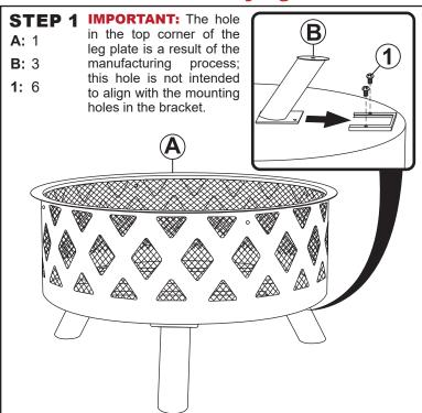
Slide three Legs (B) into the brackets on the bottom of Fire Bowl (A) and tightly secure using six M6x10mm Bolts (1).
