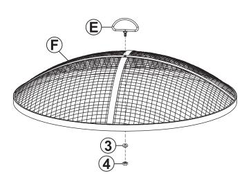
Firmly secure Spark Screen Handle (E) to Spark Screen (F) using one Washer (3) and one Nut (4).
