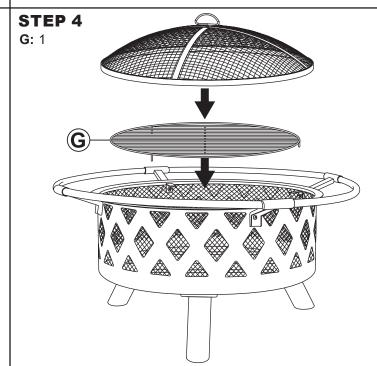
Place Wood Grate (G) into the fire bowl. Then, place the spark screen on the assembled unit.
