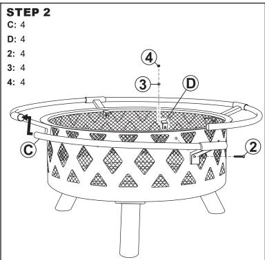
Align one Safety Ring (C) and loosely secure using one M6x20mm Bolt (2), Bracket (D), Washer (3), and Nut (4). Repeat until all safety rings are loosely secured.
