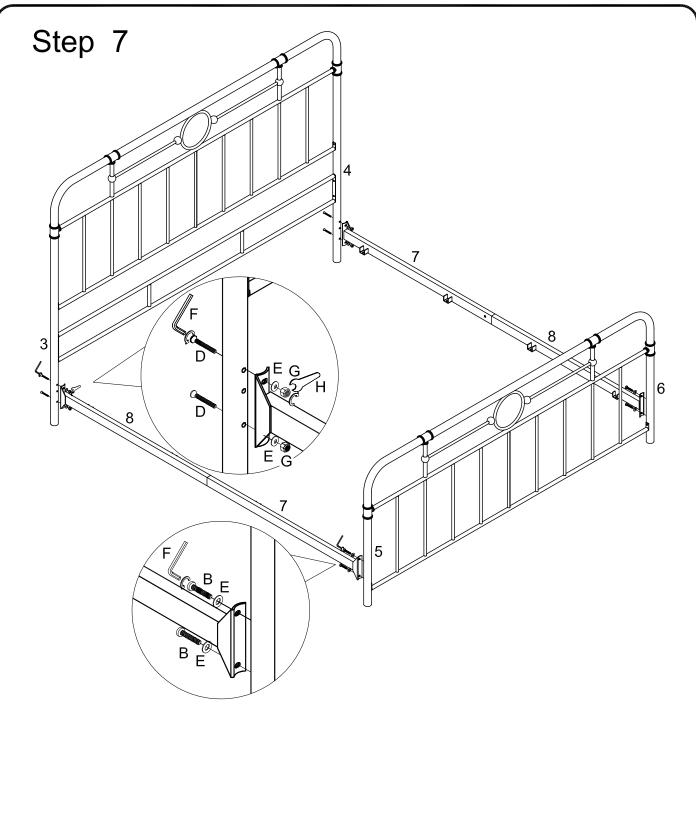
Attach part (7, 8) to part (3, 4, 5, 6) using bolt (B, D), washer (E) and nut (G) with hex key (F) and wrench (H) as per diagram.
