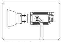
• When installing the reflector, align the reflector to the fixture's Bowens mount, rotate the reflector in the direction shown on the fixture until it clicks into place.
