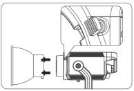
②When removing the reflector, push and hold the lock catch and rotate until the reflector is free to be removed from the fixture.
