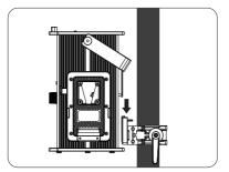
③Align the quick release plate on the control unit with the quick release mount on the clamp to mount the control unit on to the clamp.
