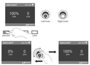
Rotate the "left knob", clockwise to increase brightness while counterclockwise to reduce the brightness. The screen shows the percentage of brightness, DIM range: 0%...100%.
