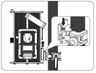
Press the lock catch on the clamp to remove the control unit from the light stand.
