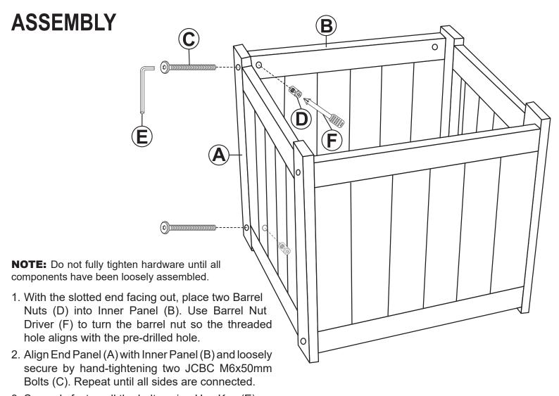
3. Securely fasten all the bolts using Hex Key (E).
