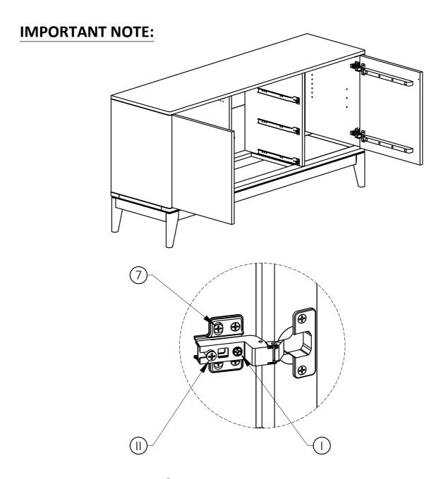
Tighten the Screw marked (I) to fasten hinge. The door may need to be adjusted so that all the spaces between the door and the unit sides are equal. To adjust, follow instructions:
