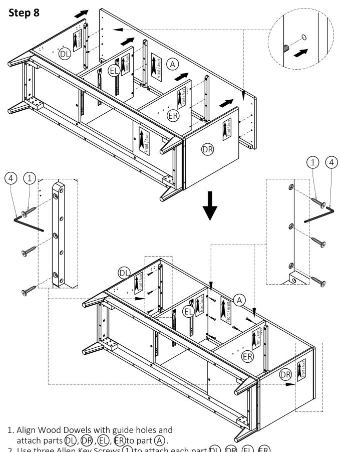
2. Use three Allen Key Screws ① to attach each part DD, DR, ED, €R through guide holes from each part DD, DR, ED, €R to pre-drilled holes of part △.
