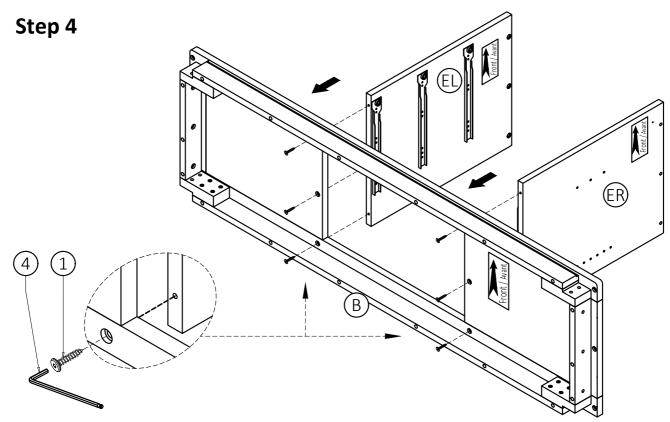
1. Use three Allen Key Screws ① to attach each part ⑥, ⑥R through guide from holes part ⑧ to pre-drilled holes of parts ⑥, ⑥R.
