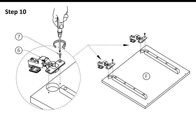
1. Attach Adjustable Hinges 6 to Doors F) using Phillips Screws 7 into pre-drilled holes on Doors F).
