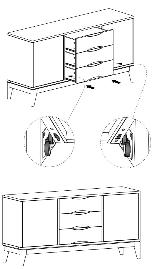
1. Insert assembled drawers into glides on assembled sideboard.
