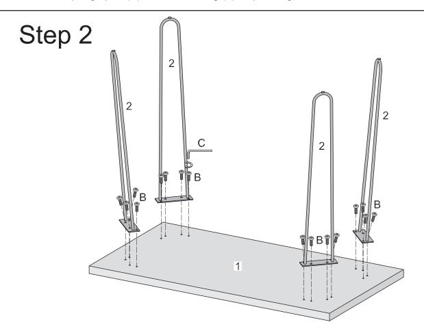
Use wrench (C), bolt (B) to secure the metal leg (2) to the table top (1).
