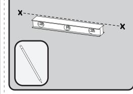
Align Mounting Plate over center point marked in previous step. Mounting Plate should be vertical as shown below. Mark Mounting Screw locations onto the wall surface. Remove item(s) after marking mounting locations.
