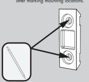
If mounting directly to wood stud, Plastic Anchors are not required. If mounting to tile, acquire proper mounting hardware capable of supporting the accessory in use. If mounting to drywall, drill guide holes at marked locations using a Drill equipped with a Ø 3/16" bit.
