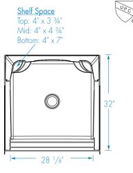
FEATURES Dimensional Tolerance ± 3/8". Dimensions needed for site preparation should be measured from the unit. Manufacturer assumes no responsibility for preparatory work.
