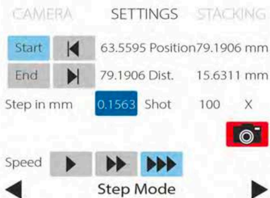
Settings Menu. Whichever mode you select, you first need to establish the start and finish point of your stack.
