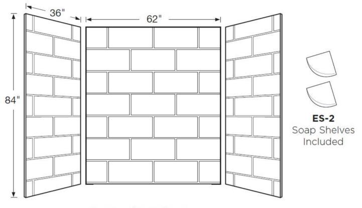
Designed to fit base areas 36" deep or smaller x 62" wide x 84" high or smaller (914 mm x 1575 mm x 2134 mm)
