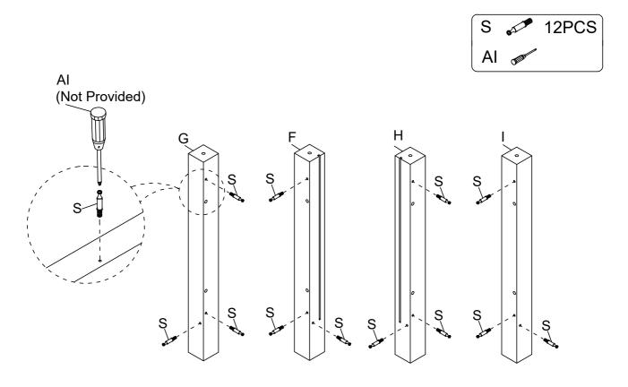
Attach two pieces of Side Panel (C) to Back Leg - Left (F), Front Leg - Left (G), Back Leg - Right (H) & Front Leg - Right (I) separately using Wood Dowel (R) by Glue (AG), then attach Nut (T) to Bolt (S) in Side Panel (C) by Screwdriver (AI) as below shown.
