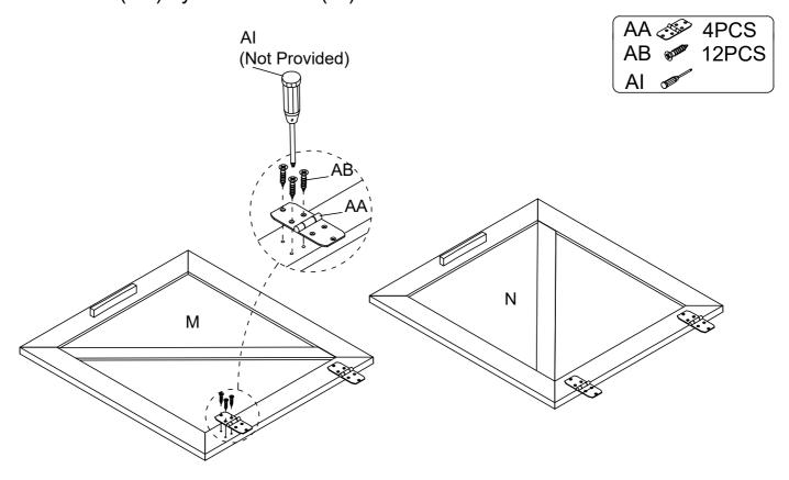
Assemble Left Door Panel (M) & Right Door Panel (N) to Front Leg - Left (G) & Front Leg - Right (I), using Hinge (AA) & Screw (AB) by Screwdriver (AI) as below shown.
