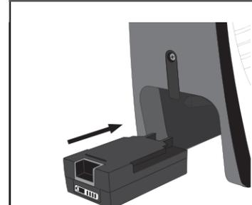
Insert Battery (until it clicks). To remove, push down on Release Button and pull away.
