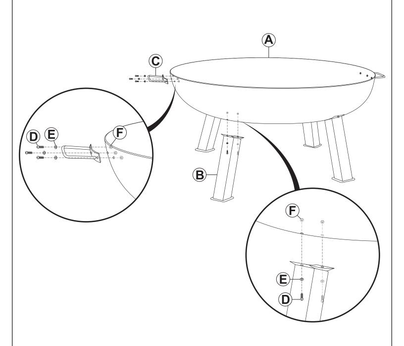
Secure one Handle (C) with the mounting holes on the side of Firebowl (A) and firmly secure using three Bolts (D), three Washers (E) and three Nuts (F). Repeat to secure the remaining handle.
