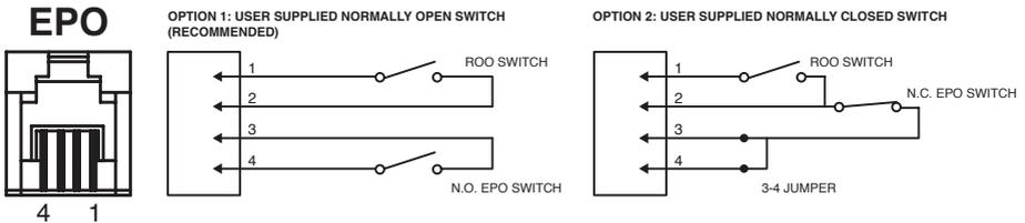
3. After wiring, make sure the external EPO/ROO switch is not activated to enable UPS output.
