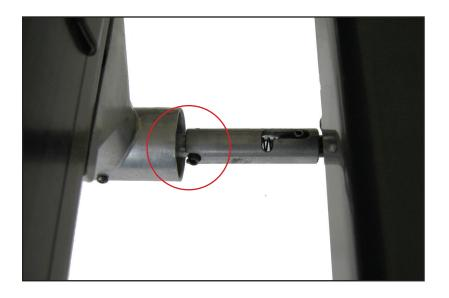
13. Make sure the slot on the spring loaded shaft engages the roll pin on the gear box.
