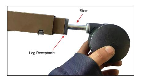
5. Install the casters by inserting the stem of the caster into the leg receptacle. It is recommended to install 1 locking caster and 1 nonlocking caster on each bed end. The locking casters should be installed diagonally from each other.
