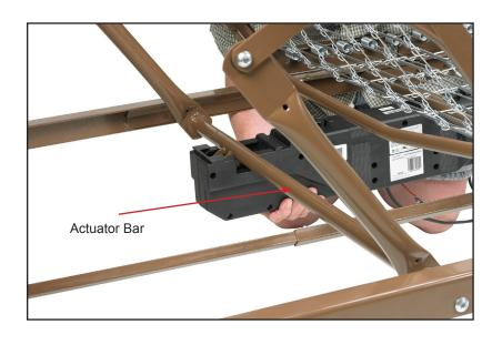
16. Align the motor with the actuator bar and lift the head spring to the highest position. The motor will automatically be pulled towards the bed and lock onto the accuator. Repeat for foot section.
