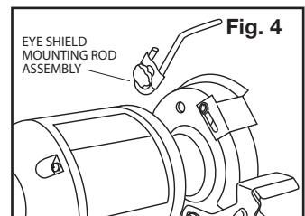
**Note:** The eye shields are identical and will fit properly on either side of the grinder. However it may be necessary to loosen the center hex nut in order to slip the shield over the mounting rod.
