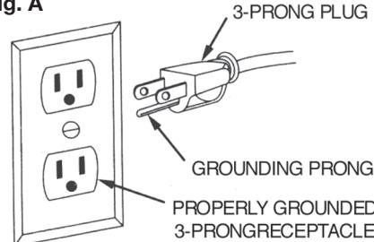
This tool is intended for use on a circuit that has an outlet that looks like the one illustrated in Figure A. The tool has a grounding plug that looks like the one also shown in Figure A. DO NOT modify the plug provided if it will not fit the outlet. Have the proper outlet installed by a professional electrician.
