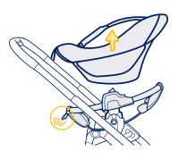
To Release Inner Carrier from Adapter
