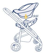
Attach the inner carrier to the inner carrier adapter. **ONLY** install the inner carrier rear-facing.
