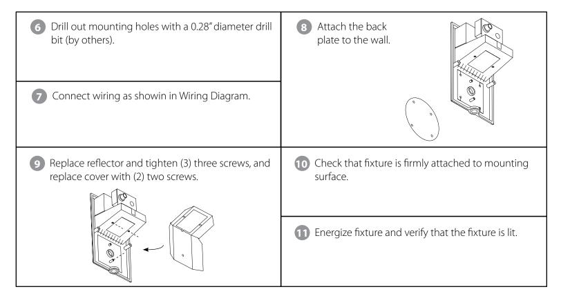
**IMPORTANT:** To weather-proof your outdoor installation, be sure to seal all mounting points, wire inlets, and penetrations (Conduit, Plugs, etc.) with silicone sealant.
