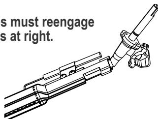
9. Attach electrode to burner.
