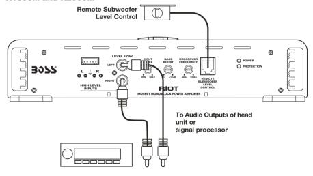
Connect the Positive (+) terminal of the subwoofer to the L (+) amplifier terminal.
