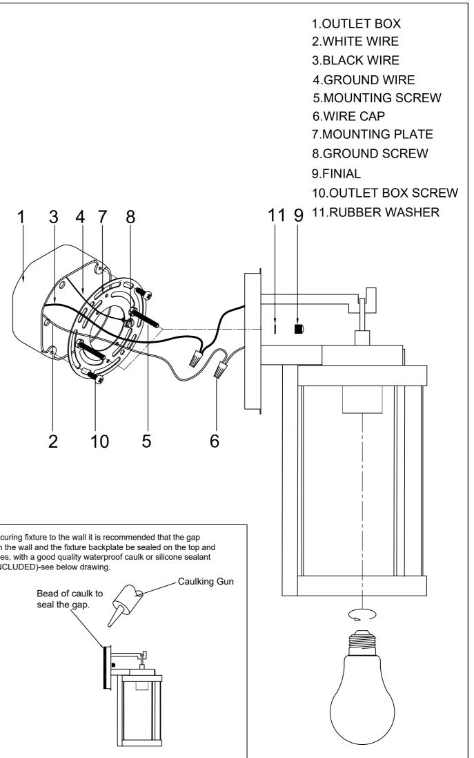
After securing fixture to the wall it is recommended that the gap between the wall and the fixture backplate be sealed on the top and both sides, with a good quality waterproof caulk or silicone sealant (NOT INCLUDED)-see below drawing.
