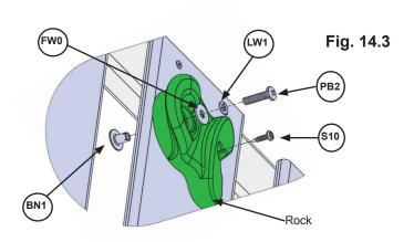
E: Place 1 rock on each (2780) Rk Board A and (2781) Rk Board B (fig. 14.2) and attach using 1 (PB2) Pan Bolt (with lock washer, flat washer and barrel nut) and 1 (S10) Pan Screw per rock. The Screw must be in the hole directly under the Pan Bolt, it will stop the rock from spinning. (fig. 14.3)
