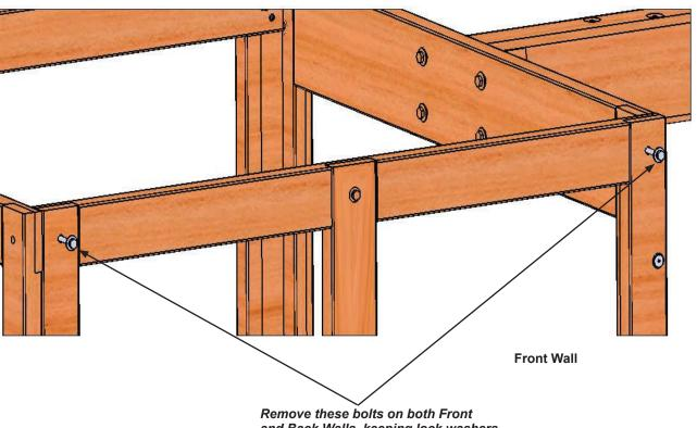
Remove these bolts on both Front and Back Walls, keeping lock washers and flat washers for next step. Do not remove the t-nuts.
