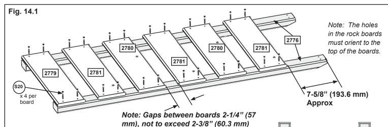
**A:** Lay 2 (2776) Rock Rails down, side by side with angled edges facing down. (fig. 14.1)
