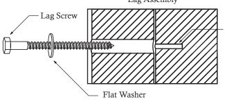
Before mounting Lag Screw, use factory drilled holes as guides to drill 1/8" pilot holes
