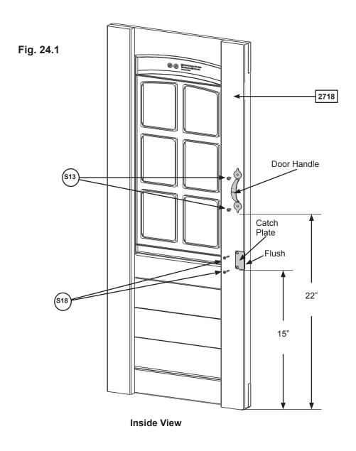
Wood PartsHardwareOther Parts1 x 2718 Door Window Panel2 x \$18 Wood Screw1 x Door Handle2 x \$13 Pan Screw1 x Catch Plate
