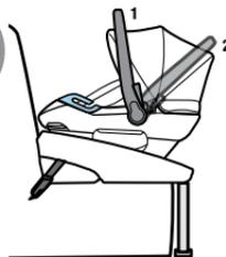
Carry Handle Must Be Locked and in Position 1 or Position 2
