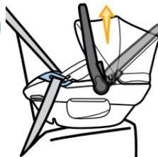
Carry Handle Must Be Locked and in Position 1 or Position 2
