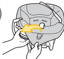
**Pull Seat Pad Down Around Bottom of Inner Carrier & Around Carry Handle Guide**
