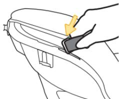
**Push Retractable Carry Handles' Metal Retainers Down Through Slots in Inner Carrier**
