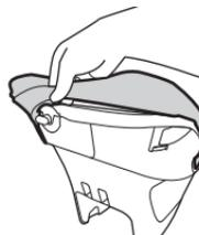
**Pull Seat Pad off of Top and Sides of Inner Carrier**
