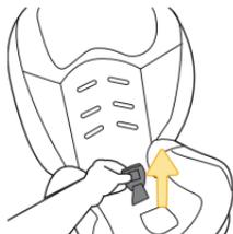
Pull Buckle Through Buckle Slot in Seat Pad
