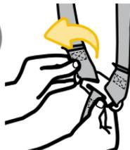
Turn Inner Carrier Over and Remove Harness Strap Loops From Splitter Plate
