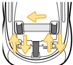
Lift Up Front of Pad and Weave Harness Strap In and Out of Shell As Shown
