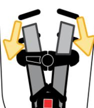
From Front of Inner Carrier, Pull Harness Straps Out of Shoulder Harness Slots
