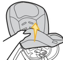
**Pull Seat Pad off of Bottom of Inner Carrier**
