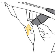
**Push Retractable Carry Handles' Metal Retainers Up into Slots in Inner Carrier**
