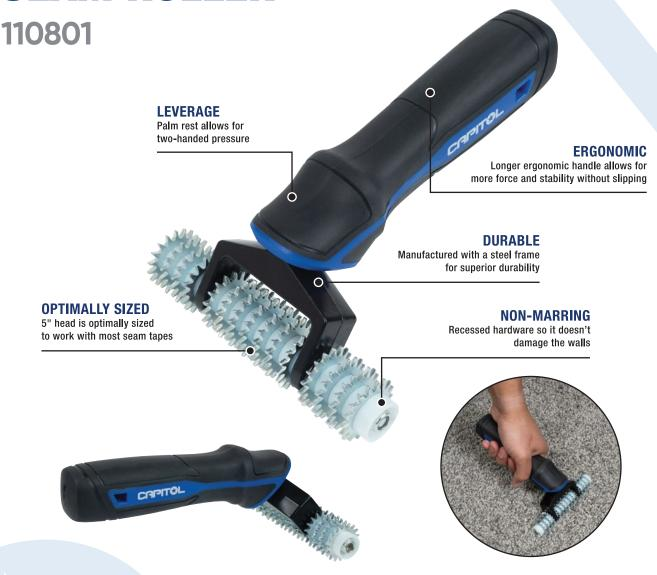
Capitol® Star Wheel Loop Pile Seam Roller is specifically designed for seaming loop pile and Berber carpets. It features star wheels to maximize the transfer of hot-melt tape into the carpet and produce stronger seams. It has a longer handle and palm rest on top of the rugged steel frame to provide optimum leverage and durability.
