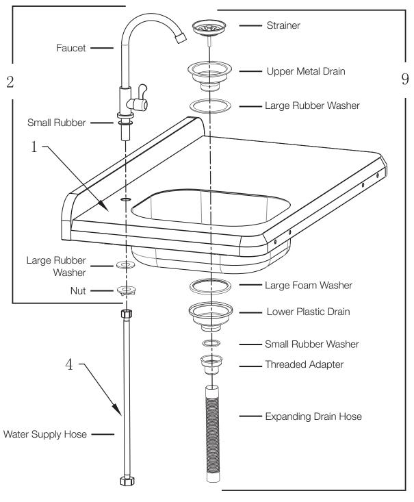
Use screw assemblies to attach the counter top assembly (1) to the prep station base. **Now tighten all screw assemblies that have been installed throughout the unit.**
