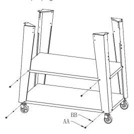
Use screw assemblies to attach name plate (15) to the left front leg (6) (LF) and the right front leg (18) (RF). Next use screw assemblies to attach the rear support to the left back leg (5) (LB) and the right back leg (17) (RB).
