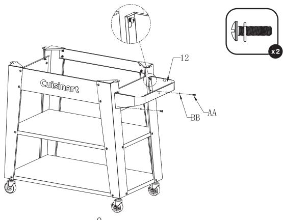
Use screw assemblies to attach both of the towel bar ends (8) to the left leg assembly.
