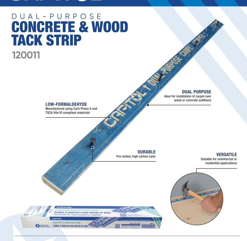
Capitol® 7/8" Dual-Purpose Tack Strip is made of 5-ply construction materials, and securely holds carpet in place with pre-nailed high-carbon nails. The pins are angled for improved gripping and to help secure the carpet after stretching. The beveled edge keeps the carpet tucked between the tack strip and the wall, and stays in place when stretching carpet with knee kickers or standard power stretchers.
