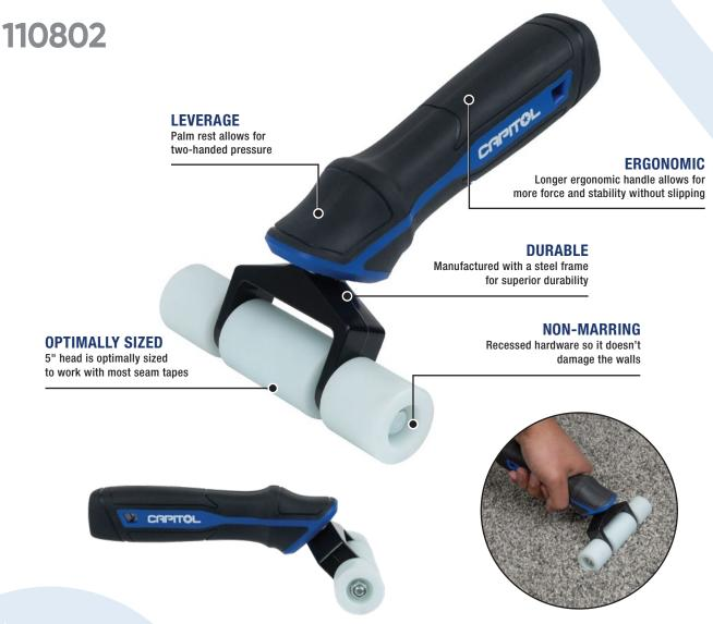
Capitol® Smooth Wheel Cut Pile Seam Roller is designed for seaming cut pile carpets, and ideal for seaming Saxony carpets as well as vinyl flooring. The soft nylon head of this roller smooths carpet without fraying yarn ends, delivering seams that have the carpet backings flush with one another, without gaps or overlays, providing a professional, finished look.
