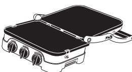
When you use the Griddler® as a Full Griddle, open the cover so it lies flat, creating a double, flat cooking surface. In this position, the foods you are preparing will have to be turned over for cooking. When using this cooking function, the griddle side of the plates should be used.
