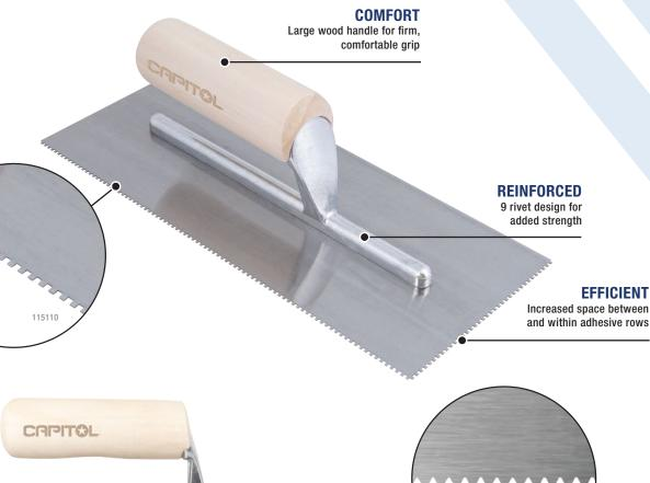
Capitol® Pro Flooring Adhesive Trowels feature a hardened, tempered steel blade for superior durability, riveted design for added strength, and square / flat-top v-notches for increased space between and within adhesive rows. Designed for professional installers, it has a large wooden handle that provides a firm, comfortable grip.
