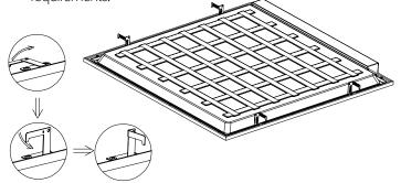
4 Remove j-box cover by removing screw. Carefully remove knockouts for line voltage and 0-10V control wires.
