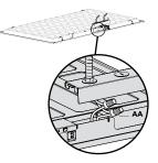
Reattach cover of junction box and secure with screw.
