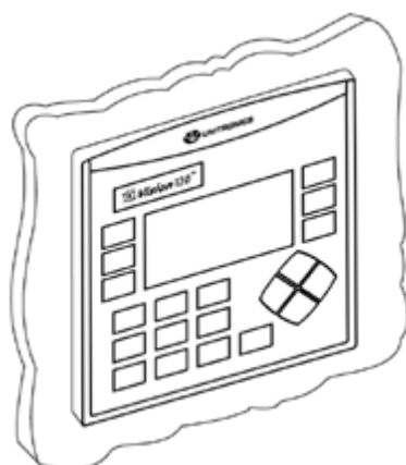
Figure B-9. Remote Relay Panel Mounted
