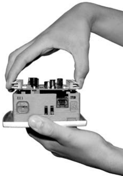
Figure B-7. Remote I/O Printed Circuit Board Removal
