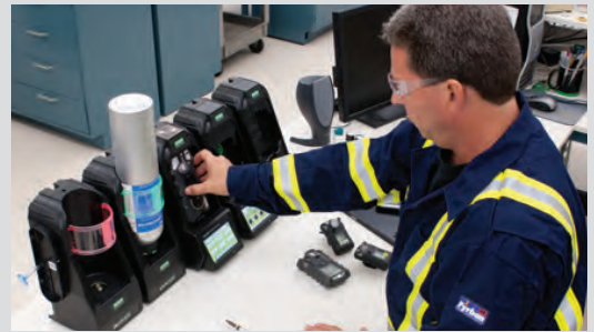
MSA's GALAXY® GX2 Automated Test System offers ease of use, reduced cost of ownership and proactive safety management. Integrated system provides simple and intelligent testing and calibration of MSA ALTAIR® product family.
