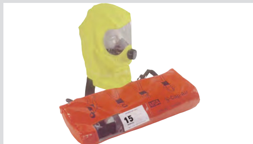
The S-Cap Air is a compressed air, constant flow, escape breathing apparatus designed to aid escape from hazardous areas in which toxic substances or oxygen deficiency may occur.
