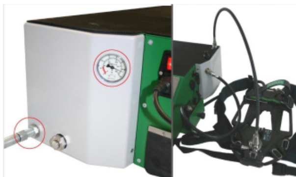
Figure 26 Connecting high pressure line
