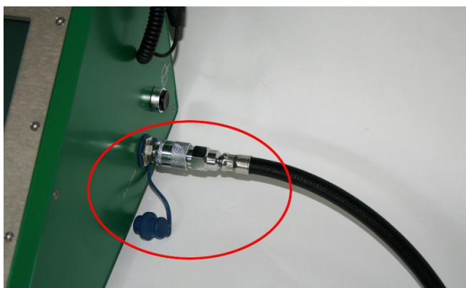
Figure 19 Connecting medium pressure line
