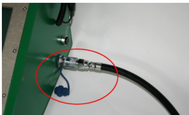
Figure 25 Connecting medium pressure line
