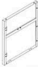
S14 CABINET SIDE PANEL ASSEMBLY - A4M04536 (x1) 26 9/16"x23 3/8"x1 3/8" (35x594x675)
