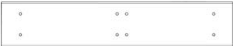
OG01 FLOOR JOIST - W4L22461 (x2) 1 3/16"x3 3/8"x17 1/4" (30x86x438)
