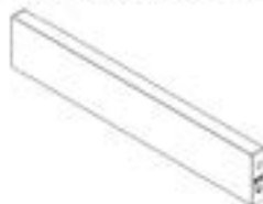
A4 SINK CABINET HORIZONTAL CHANNEL - A4M03097 (x2) 1"x3 3/8"x18 3/8" (25x85x466)
