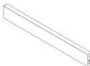
A1 CORNER CABINET HORIZONTAL BEAM ASSEMBLY - A4M03032 (x2) 1"x2 3/4"x22 1/4" (25x70x565)
