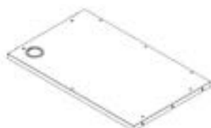
T2 GRILL TABLETOP ASSEMBLY - A4M03057 (x1) 1 1/4"x23 3/8"x38 3/16" (32x594x970)
