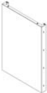
S4 SINK CABINET SIDE PANEL ASSEMBLY R - A4M03093 (x1) 2 5/8"x23 3/8"x33 3/8" (67x594x848)
