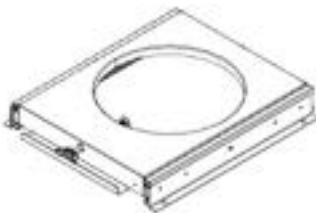
A13 GAS TANK HOLDER ASSEMBLY - A4M03047 (x1) 1 15/16"x12 7/8"x14 3/4" (49x327x374)
