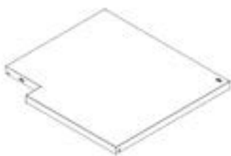
C4 CORNER CABINET SHELF ASSEMBLY R - A4M03046 (x1) 1 1/4"x23 1/8"x25 7/16" (32x588x646)
