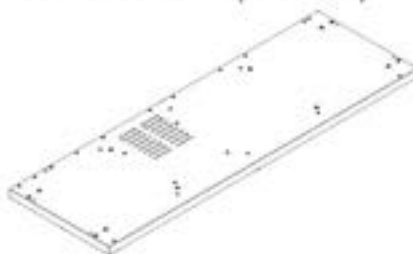
F4 PIZZA OVEN CABINET FLOOR PANEL ASSEMBLY - A4M03062 (x1) 2 5/8"x23 3/8"x72 3/16" (66x594x1834)
