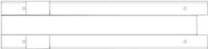
OG08 WIREWAY BOARD - W4L22040 (x1) 1 3/16"x3 3/8"x14 7/16" (30x86x367)
